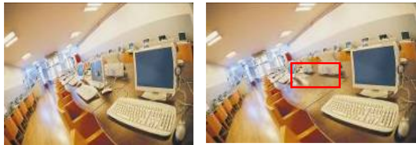
On-board analytics can detect meaningful changes in sequential video clips and trigger alarms. In the scene pictured above, a PC has been removed from the table (right).
